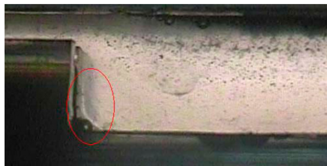
Fig. 7. Stress frozen fringe in the cavity using 10% HPC.
