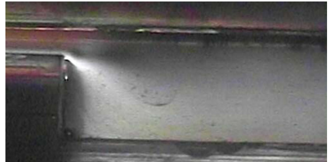
Fig. 5. Showing the fringe pattern observed the cavity using 7% concentration of HPC in a dark field polariscope.
